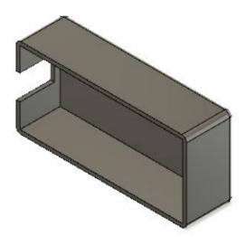
This case is used protect the micro-controller from yhe external environment. The grove is used for connecting the micro-controller to power supply.
